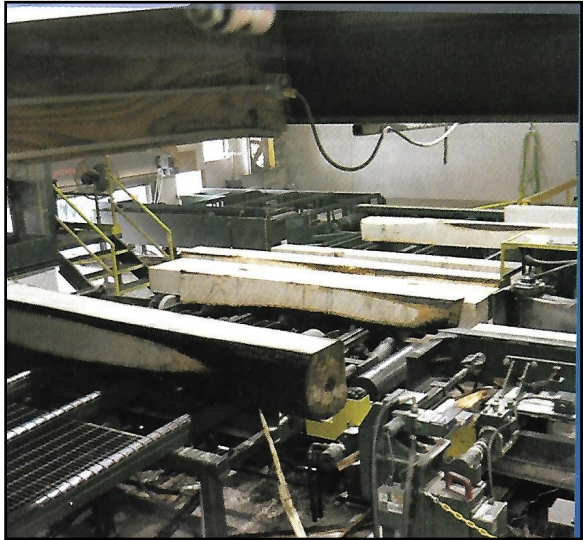
Cants, boards sawn into dimensions thicker than three inches by standard width, enter Kretz's pallet factory. Lumber not kiln-dried is shipped to pallet and railroad tie manufactures.
