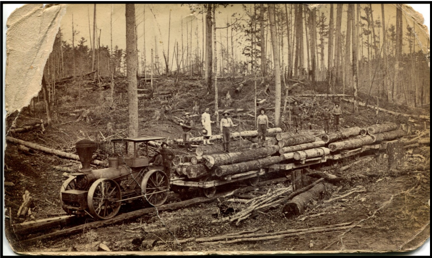
Traction and Tramroad Engine, Patented by E.P. Cowles, Wequiock, Brown County, Wisconsin. (W. H. Upham Collection, North Wood County Historical Society, Marshfield., Wisconsin.)
