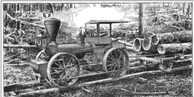
FIG. 8.—COWLES' PATENT LOCOMOTIVE FOR POLE ROADS. Constructed by Messrs. SPANGENBERG, PENDLETON & Co., Warren, Ohio.
