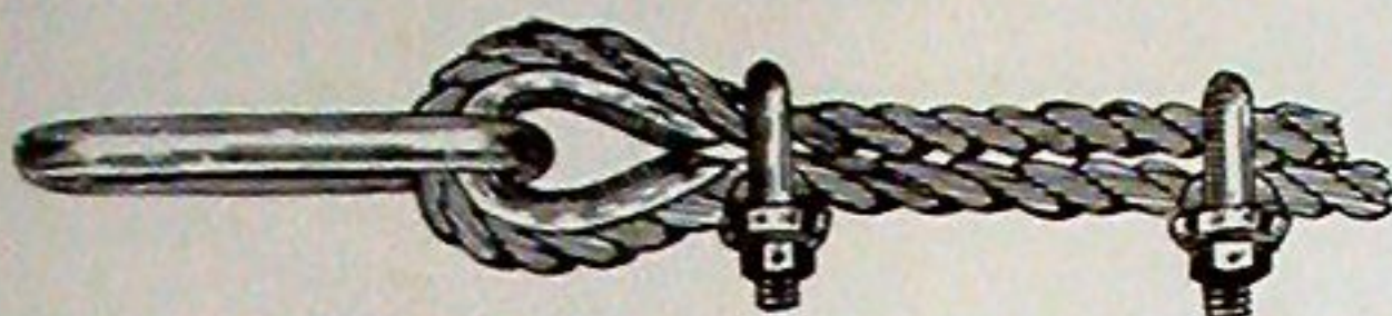
Method of attaching Wire Rope Thimbles and Clips
