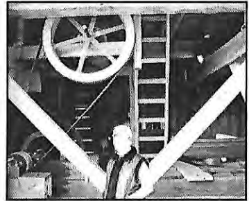
The drive belts and wheels for the waterpowered sawmill at Wade House
