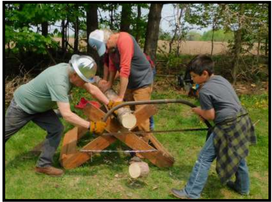
The Kids learned that a two man Saw Team learned to only "pull" on the saw to a point the partner pulls back. The weight of the saw is the only down pressure---or the saw will 'jam'.
