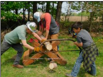
The kids learned that a two-man saw team should only pull the saw—never push it—and each partner pulls in turn. The weight of the saw provides all the downward pressure; adding more will cause it to jam.
